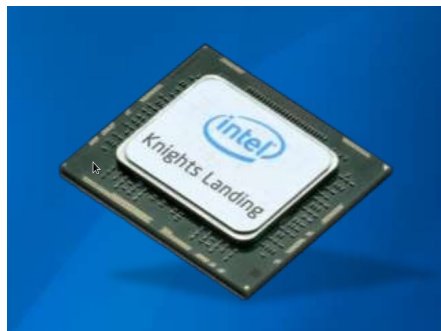
Figure 1.22: Second generation MIC processor codenamed Knights Landing will be available in the socket version (i.e., as a stand-alone CPU).
