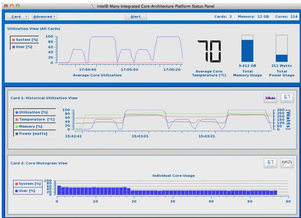
Figure 1.26: The GUI mode of the micsmc tool illustrating the execution of a workload on a system with two Intel Xeon Phi coprocessors.
