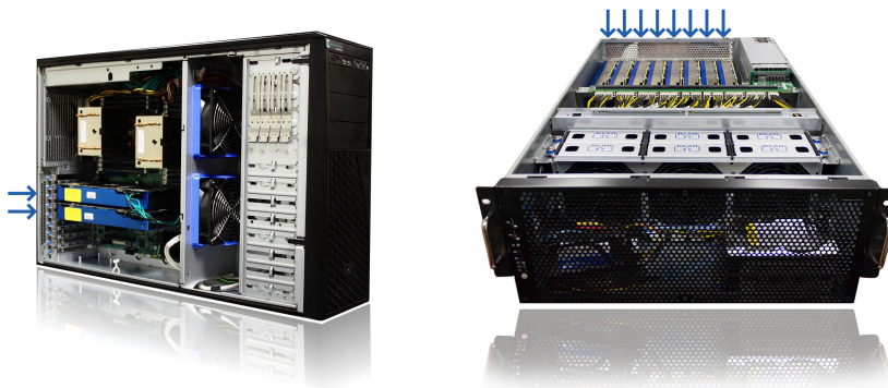
Figure 1.2: Examples of computing system solutions featuring the Intel Xeon Phi coprocessors. Left: A Colfax Workstation CXP7450 with two Intel Xeon Phi coprocessors. Right: A Colfax Server CXP9000 with eight Intel Xeon Phi coprocessors. Relative sizes not to scale.
