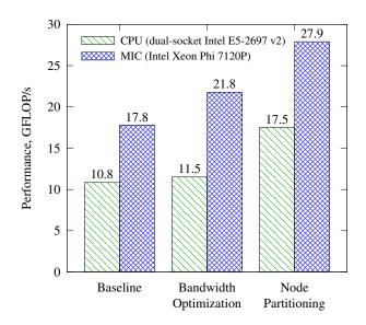
**Figure 2:** Single-node performance: dual-socket Intel Xeon E5-2697v2 processor and Intel Xeon Phi 7120P coprocessor. See Section 3 for discussion.
