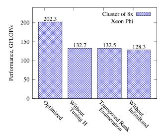
**Figure 4:** Tuned performance and degraded performance of eight Xeon Phi coprocessors in two compute nodes of the cluster. See Section 4 for discussion.
