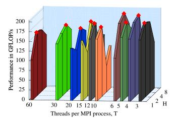
Figure 5: Two parameters must be empirically determined for each problem size N and cluster size M: (i) T, the number of threads per process, and (ii) H, the number of blocks in the x-dimension for grid partitioning. The best-performing pair of (T,H) can then be used in production runs. Shown are results of calibration for N=10000, M=8. Red markers indicate the best values of H for a given T.
