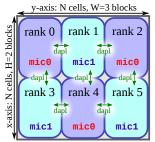
Figure 6: Rank assignment in a grid of  $R=W\times H$  processes. Left: optimized rank enumeration with the :ppn suffix in the machine file (Listing 7). Most left and right neighbors are local (on the same coprocessor) and communicate via the shared-memory copy protocol shm. Right: sub-optimal rank enumeration with the -np=R argument of mpirun (Listing 8). All left/right and top/bottom neighbors are remote, communicating via the InfiniBand protocol dapl.
