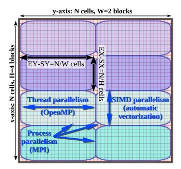
Figure 1: Simulation domain of  $N \times N$  cells is partitioned into H blocks x-wise and W blocks y-wise, and each block is assigned to an MPI process. Within each MPI process, OpenMP is used to distribute iterations in the y-dimension between threads, and automatic vectorization is applied in the x-dimension.
