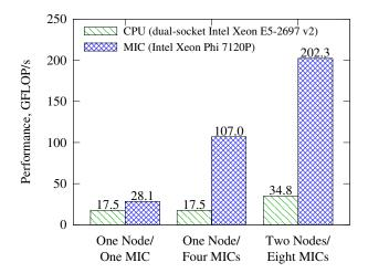
**Figure 8:** Scalability across multiple coprocessors and multiple CPUs. In this plot, the second and third set of bars show the performance achieved within the same rack space with only CPUs and only MIC accelerators (one node in the second set of bars and two nodes in the third set).
