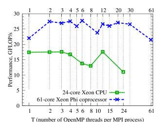
Figure 3: Impact of node partitioning between several MPI processes on performance. Data obtained on the host and on the coprocessor. In each run, the number of MPI processes is chosen as 24/T on the CPU, and as 61/T on the coprocessor (with rounding).
